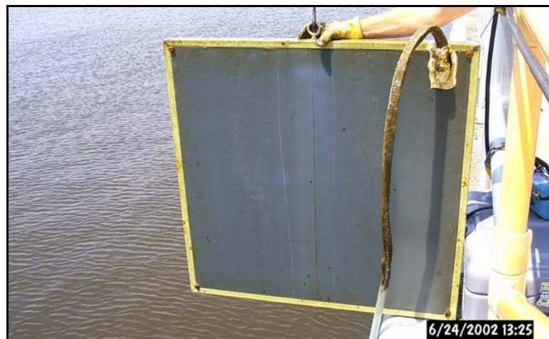
a. EES “live” panel raised out of water for first periodic inspection.
