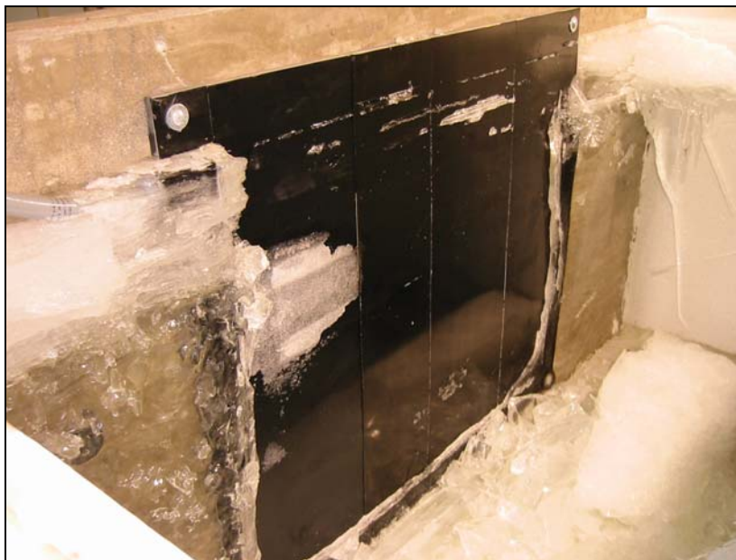
b. Panel clear of ice (except for the white patch of frost near left center) after only four firing cycles.
