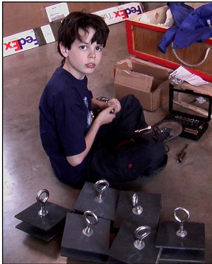
a. Assembling sets of small plates, one each of which was retrieved monthly and returned to the laboratory for sampling.
