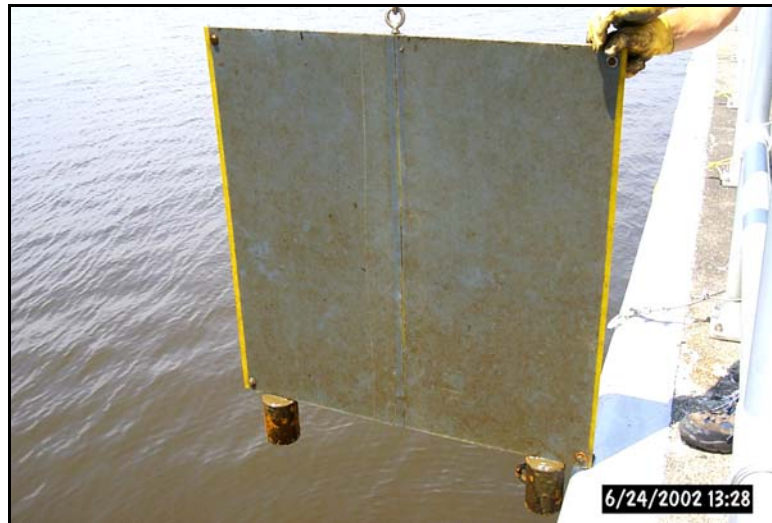
b. EES “control” panel raised out of water for first periodic inspection.
