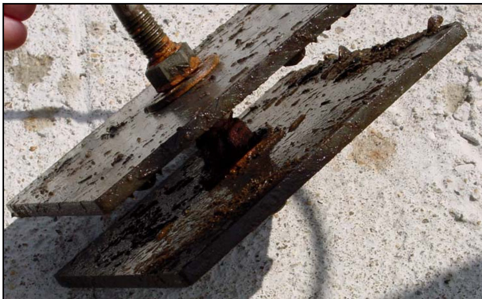
b. Set of small plates retrieved from the water, showing zebra mussels attached along the right-hand edge.
