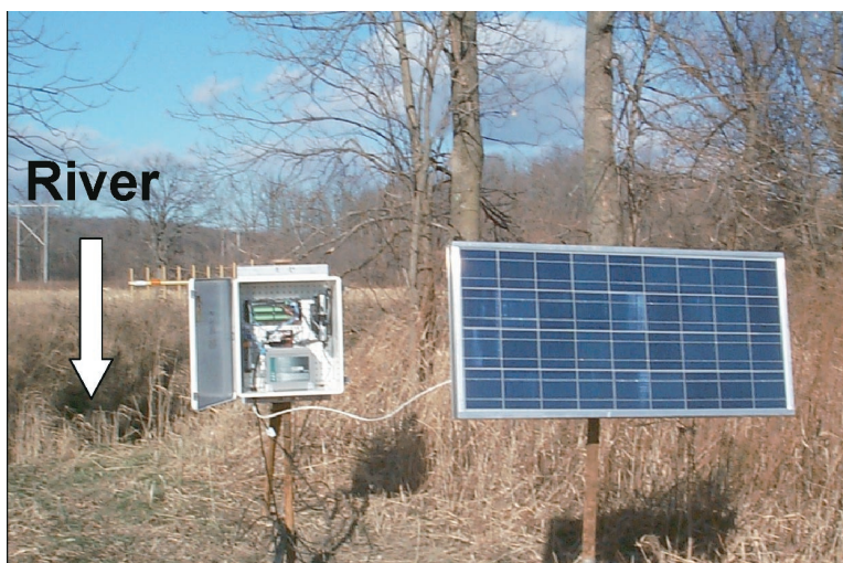
Figure 1. Data acquisition system and solar cell on bank of LaPlatte River, Hinesburg, VT
