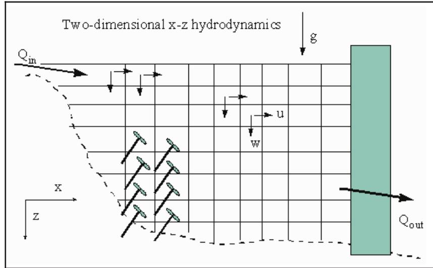
Figure 1. Typical CE-QUAL-W2, Version 2 model grid
