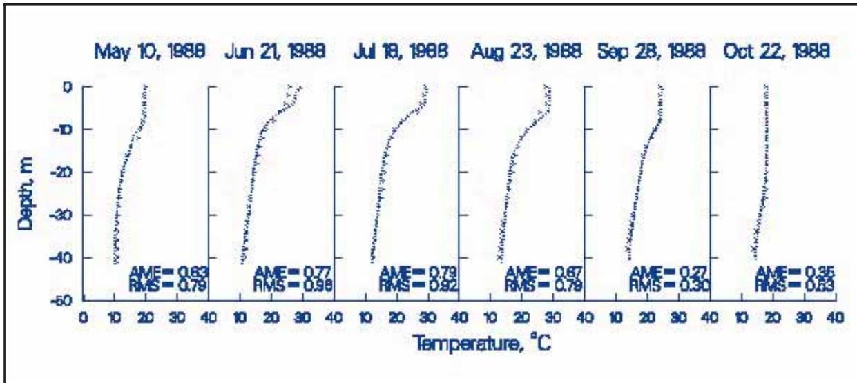
Figure 7. 1988 JST computed versus observed temperature
