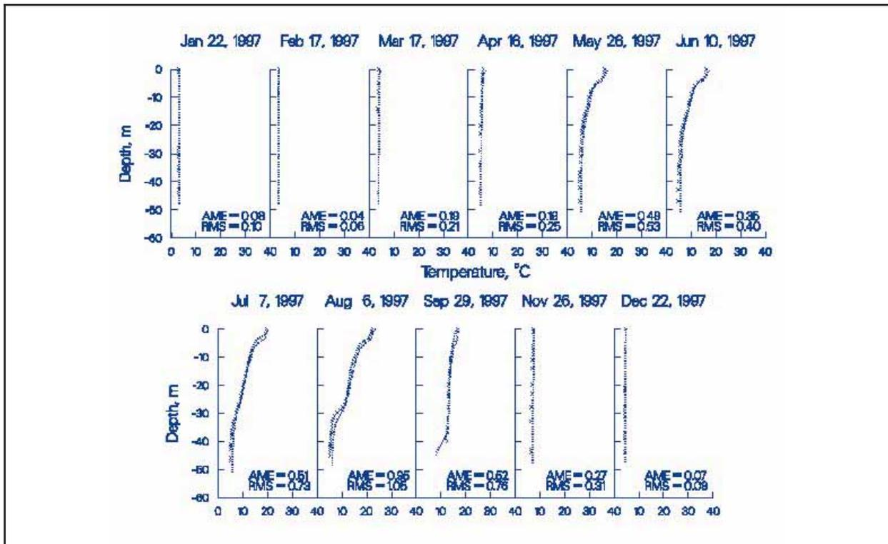
Figure 26. 1997 Bull Run Reservoir 1 computed versus observed temperatures
