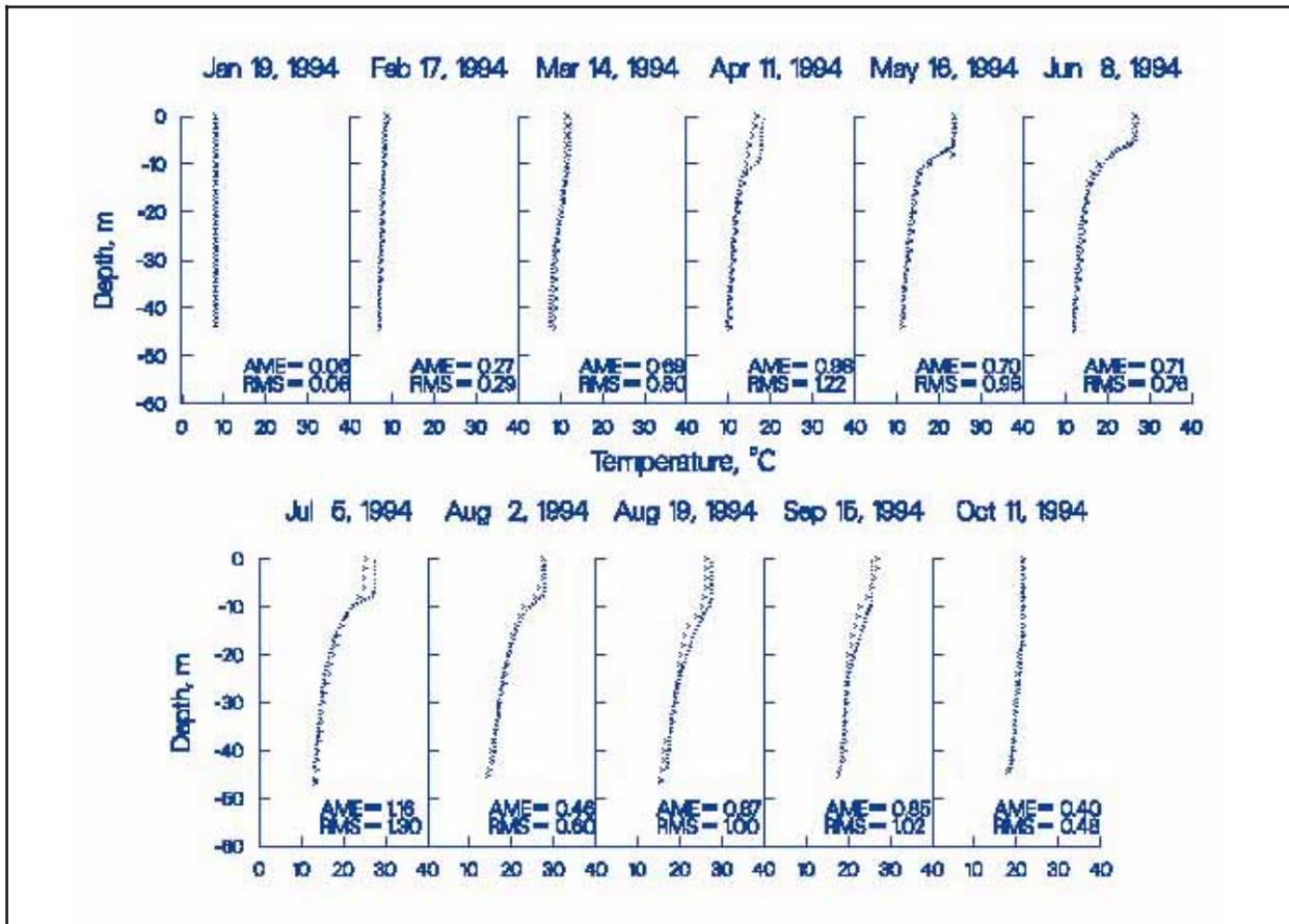
Figure 8. 1994 JST computed versus observed temperature
