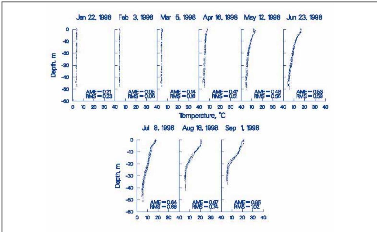
Figure 27. 1998 Bull Run Reservoir 1 computed versus observed temperatures
