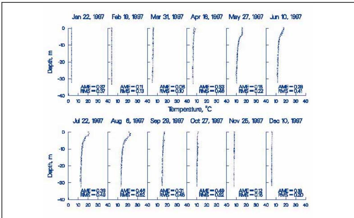
Figure 28. 1997 Bull Run Reservoir 2 computed versus observed temperatures
