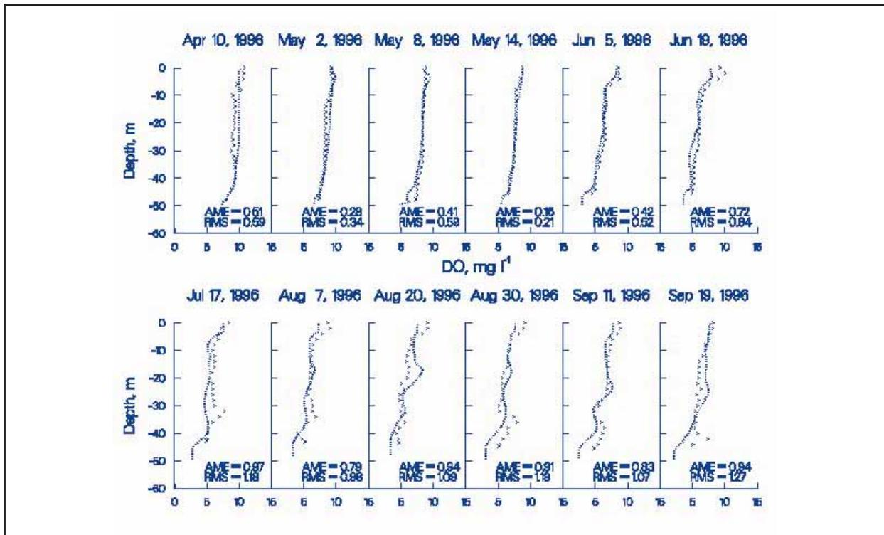
Figure 13. 1996 RBR computed versus observed DO
