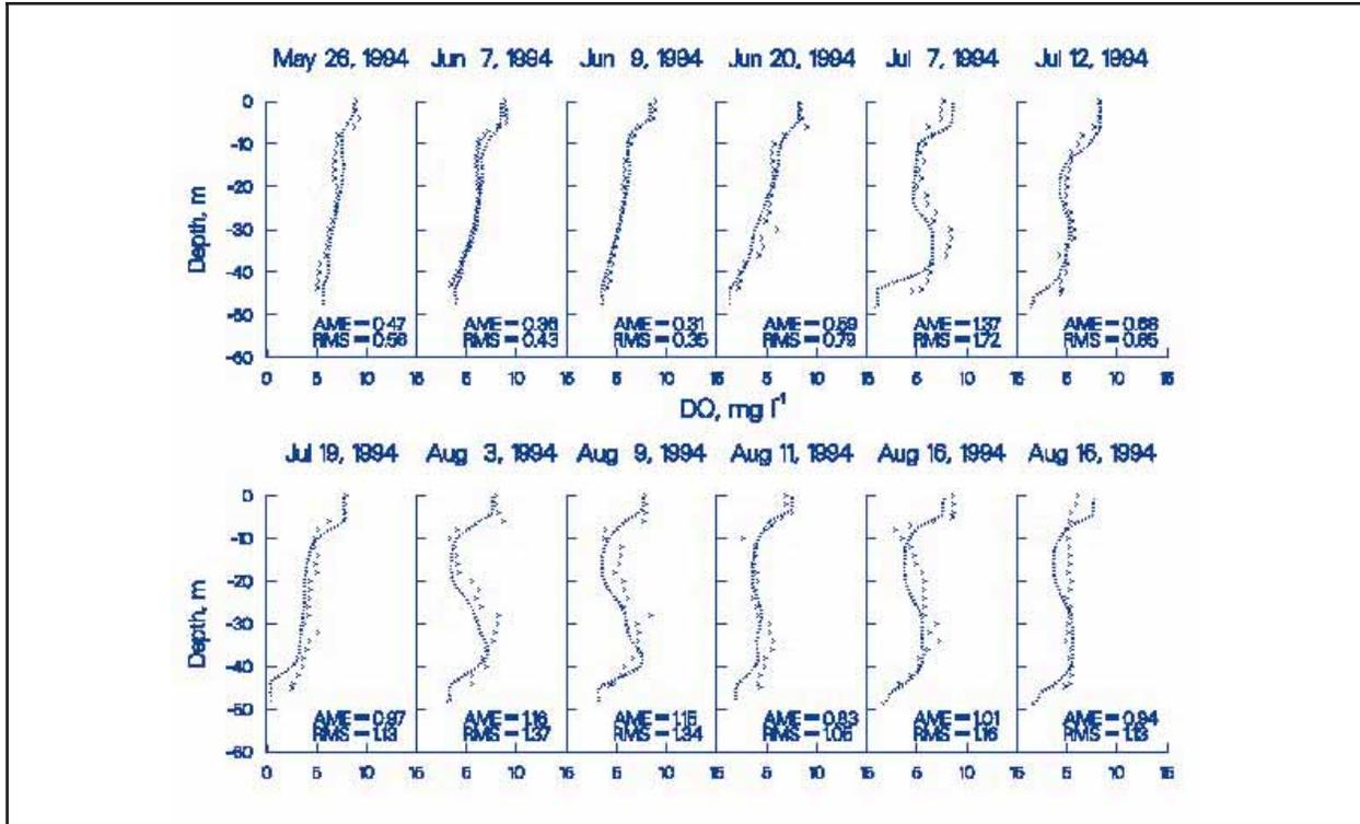
Figure 12. RBR 1994 computed versus observed DO
