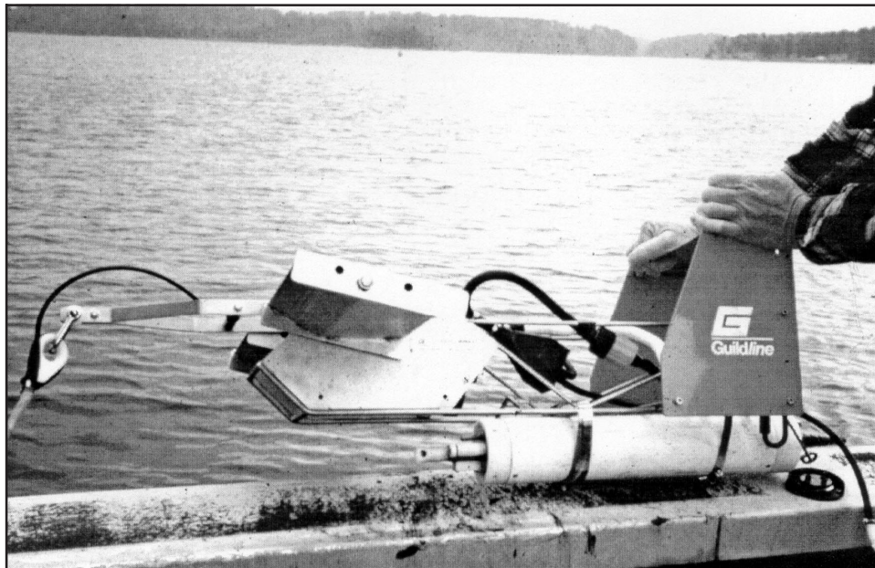
Figure 6. The Guildline MiniBAT® with Hydrolab water quality sonde attached
