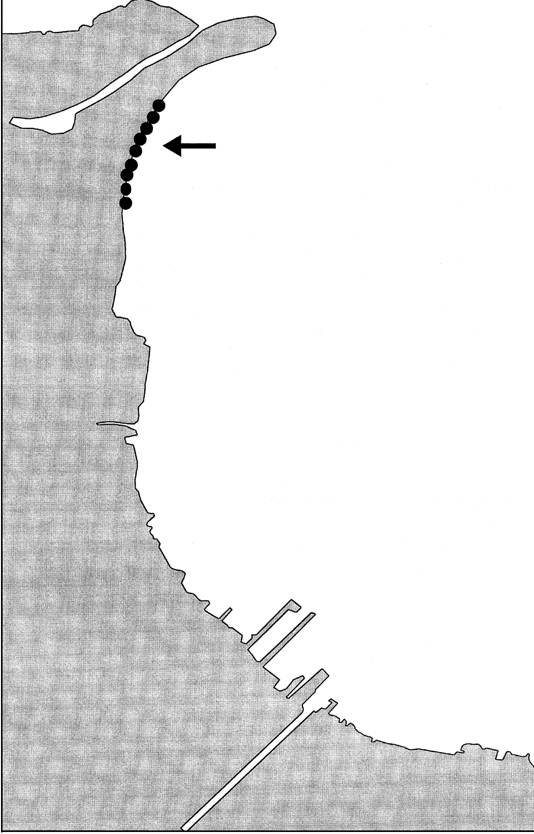
Figure 52. Sampling station locations along the Metro Beach area during the dye dissipation study on 25 August 1998. Arrow identifies the sampling station used to determine residence time of the nearshore beach area
