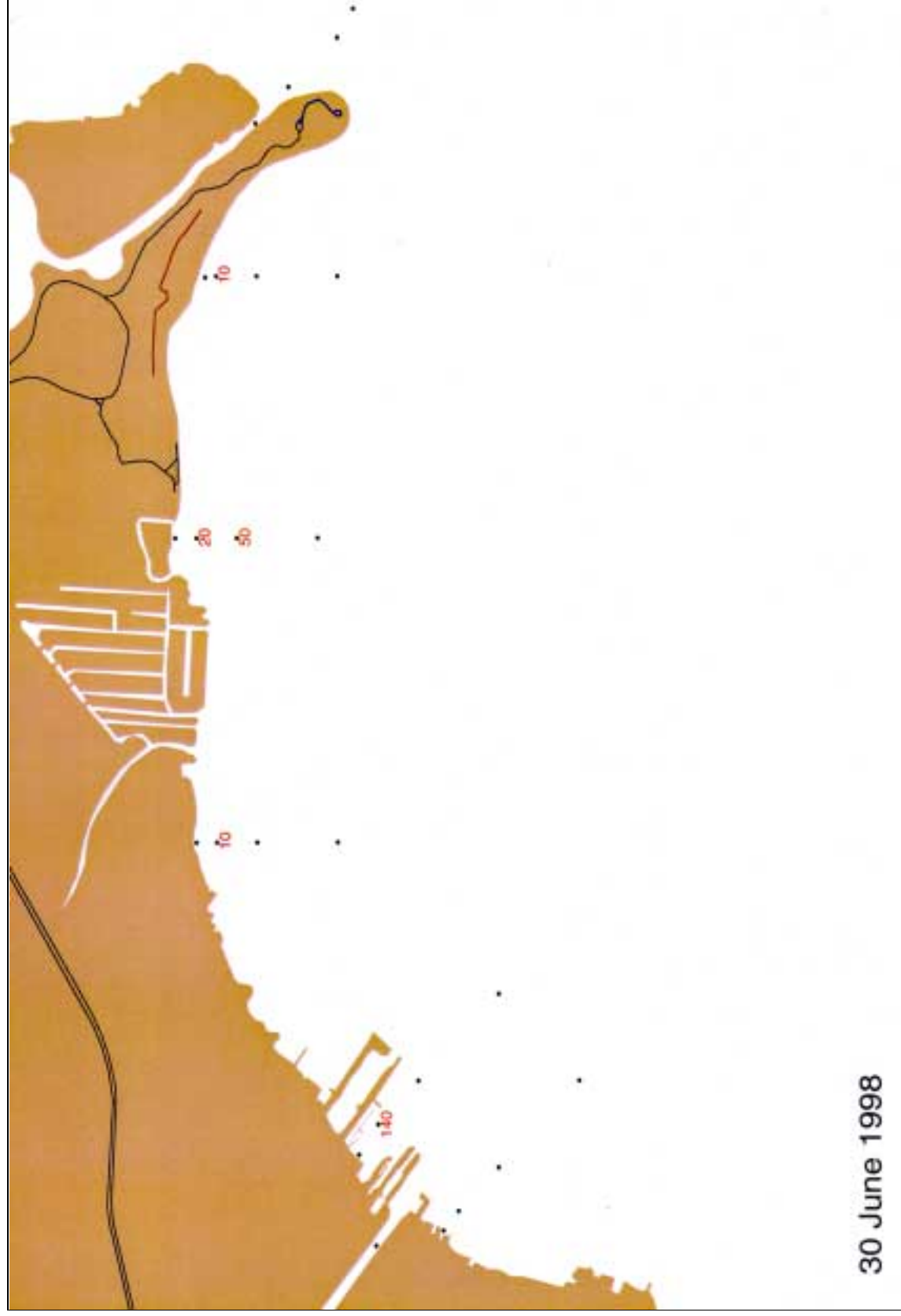
Figure 11. Concentrations of fecal indicator bacteria measured on 30 June 1998. Numbers indicate E. coli counts at the adjacent sampling point. Unlabeled sampling points had E. coli concentrations below the detection limit
