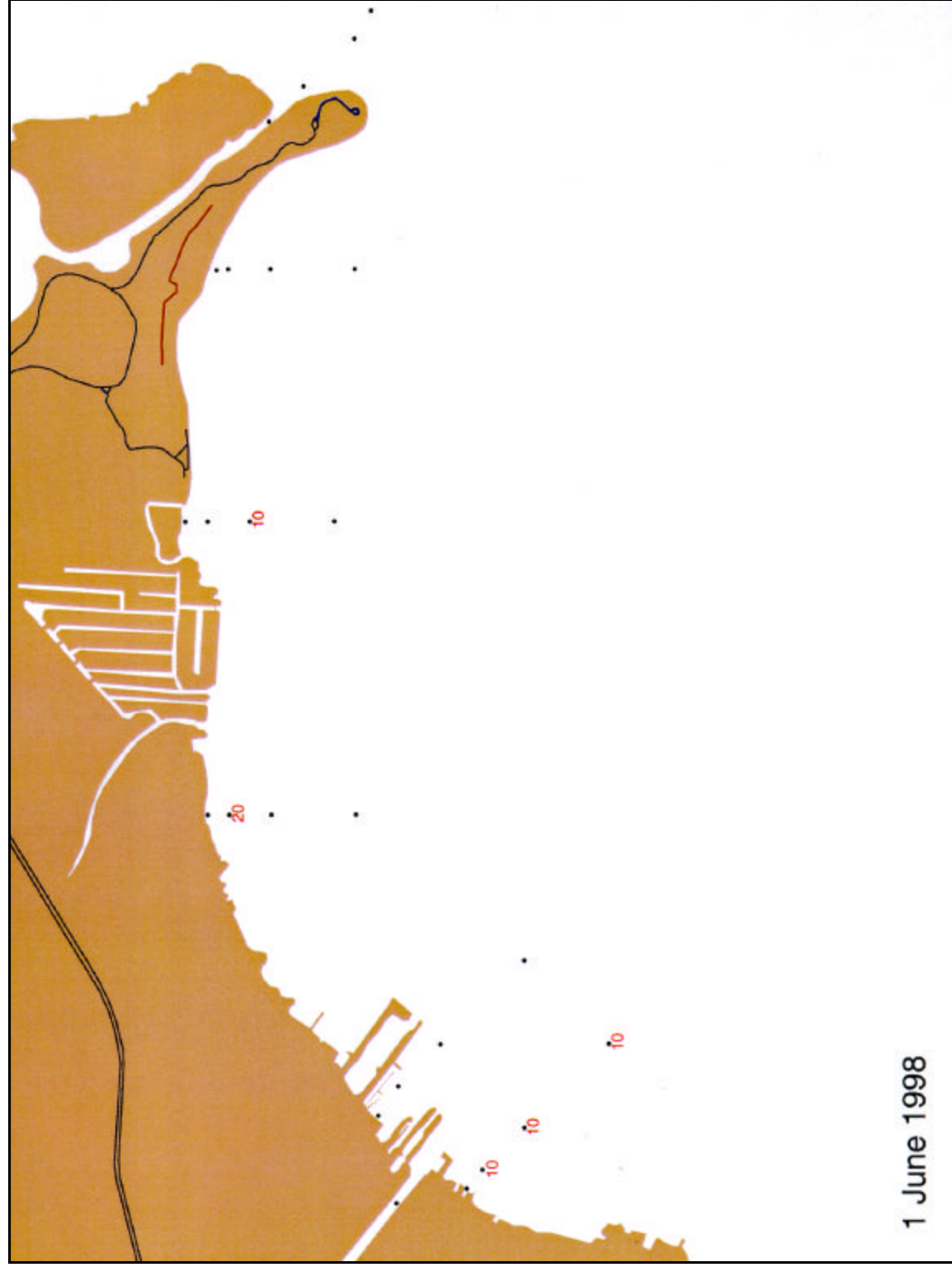
Figure 10. Concentrations of fecal indicator bacteria measured on 1 June 1998. Numbers indicate E. coli counts at the adjacent sampling point. Unlabeled sampling points had E. coli concentrations below the detection limits
